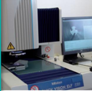
Developing and manufacturing new products is the first part, measuring is the second. To be able to measure tolerances within thousands of a millimetre, we have at our disposal an optical measuring device. This of course is the latest and highest standard in measuring equipment.
